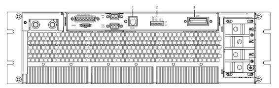
Figure 3-1. SG Unit with GPIB/RS232 Option
