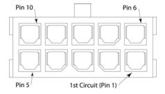
Figure 5-7. External User Connector (rear panel view) Designation (10-pin Molex)
