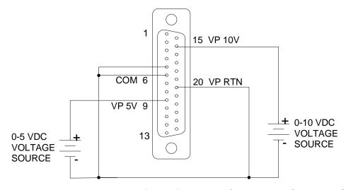
Figure 7-5. Remote Voltage Programming Using 0-5 VDC or 0-10 VDC Voltage Source
