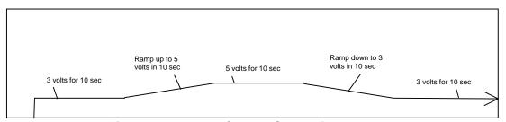
Figure 6-1. Power Supply Output for Example 1
