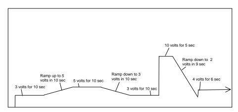
Figure 6-3. Power Supply Output for Example 3
