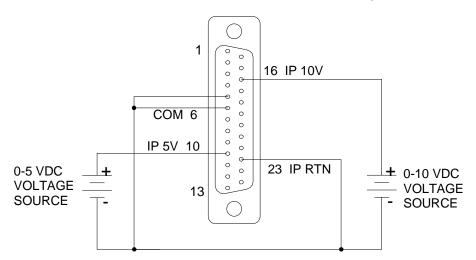
Figure 7-3. Remote Current Programming Using 0-5 VDC or 0-10 VDC Voltage Source
