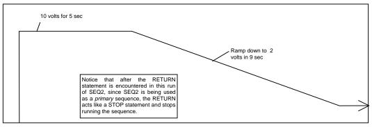
Figure 6-2. Power Supply Output for Example 2
