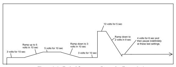
Figure 6-4. End-of-Sequence Pause for Example 4
