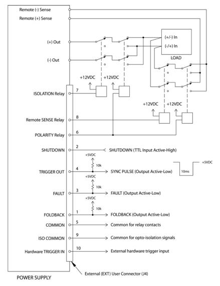
Figure 5-8. Example of Open Collector, TTL Input, and Relay Output Circuits
