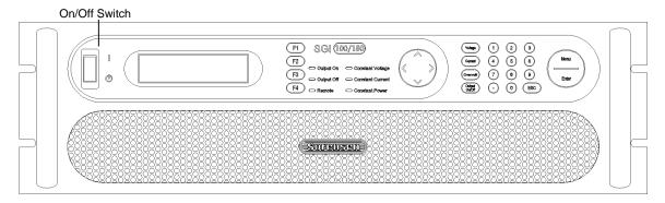
Figure 7-4. SGI Front Panel
