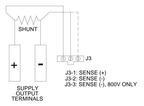
Figure 7-2. Precision Current Shunt
