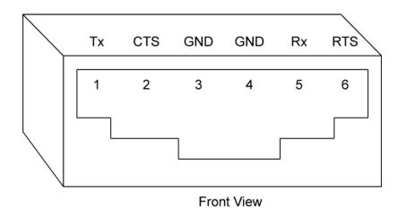
Figure 3-8. RS232 Rear Panel RJ-11 Connector Pinout
