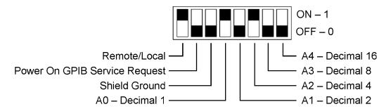
Figure 3-5. SGA Configuration Switch for GPIB
